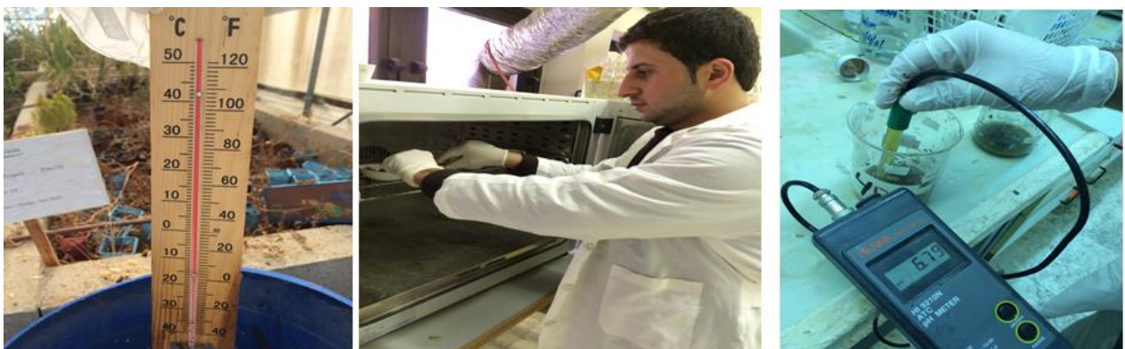
Figure 3-4: Monitoring moisture content, pH and temperature
